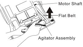
Place a new flat belt onto the motor shaft and pulley.
